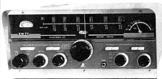
The KW Triple Conversion Super with many refinements
