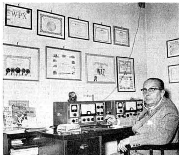
ITIAGA of Palermo, Sicily, has made nearly 33,000 QSOs since March, 1952, and is the holder of 224 operating awards. His transmitter runs 60 watts input and the aerial is a Windom.
